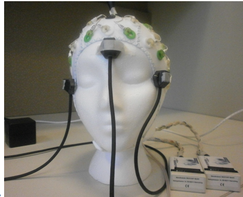
Electrode position measurements via Polhemus Fastrak 3D Digitizer System
