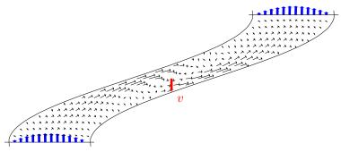
Left&right boundary: zero flow. Bottom resp. top: flow in resp. out.
