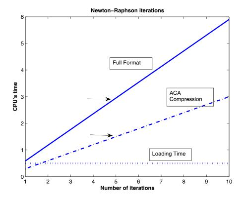
Figure 3.4: Comparison of loading CPU time (dotted line), calculational CPU time for the full-format N-scheme (solid line) and ACA-based N-scheme (dash-dotted line) with respect to the number of iterations. The arrows depict the time when the demanded accuracy is achieved.
