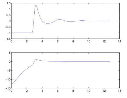
Figure 1.1: Radial parts of correlation functions h(r) (top) and c(r) (bottom) of a simple mono-atomic liquid with density  $\rho = 0.7$  and Lennard–Jones potential parameter  $\varepsilon = 0.7$ .
