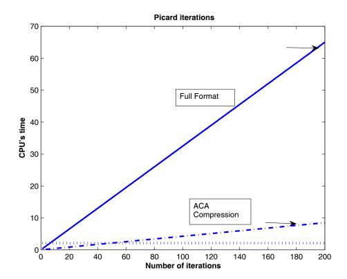
Figure 3.3: Comparison of loading CPU time (dotted line), calculational CPU time for the full-format Picard scheme (solid line) and ACA-based Picard scheme (dash-dotted line) with respect to the number of iterations. The arrows depict the time when the demanded accuracy is achieved.
