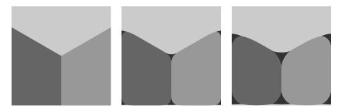
Figure 12: Nucleation and growth of a fourth phase in the evolution computed by Algorithm (42-45), even though the initial condition contains only three phases, and the surface tensions satisfy the triangle inequality. Leftmost panel shows the initial condition.
