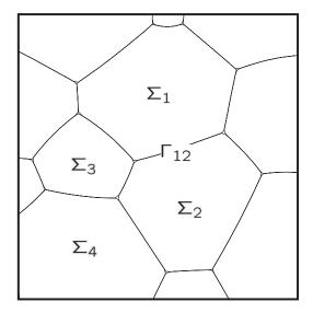
Figure 1: A partitioning of a domain into sets  $\Sigma_j$  that intersect only at their boundaries. Interface  $\Gamma_{i,j}$  separates  $\Sigma_i$  from  $\Sigma_j$ . This set-up appears e.g. in materials science, where the sets  $\Sigma_j$  represent grains (individual single-crystal pieces) making up a polycrystalline material
