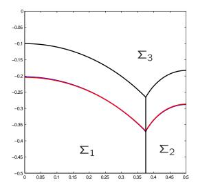
Figure 8: Numerical convergence test against an exact, travelling wave solution. The initial condition is the configuration of black curves. The blue curves are the computed solution (on a  $1600 \times 1600$  grid) and the red ones are the exact solution, at time t = 0.096. The angles at the junction are  $(135^{\circ}, 150^{\circ}, 75^{\circ})$ .
