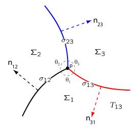
Figure 2: The angles  $\theta_j$  formed at a triple junction p are determined according to formula (7) by the surface tensions  $\sigma_{i,j}$  of the interfaces meeting there. The tangent to the triple curve points into the page in this picture.
