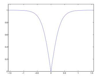
Figure 6: According to Read & Shockley [32], the typical dependence on the misorientation angle  $\theta = \min_{k \in \mathbb{Z}} |\theta_i - \theta_j + k\pi/2|$  of the surface tension  $\sigma_{i,j}(\theta)$  associated with a grain boundary formed between two planar grains with cubic lattices.
